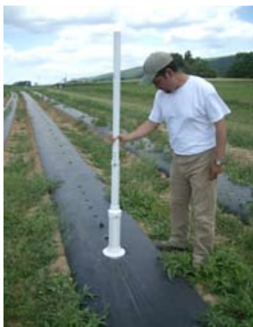
Figure 2. Manual hand-held dibbler in use on a plastic mulch covered raised bed.
