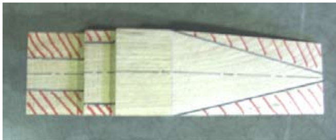
Figure 6. Block of wood (l) for cone-shaped dibble tip marked for cutting in second plane (use dimensions of figure 5a).
