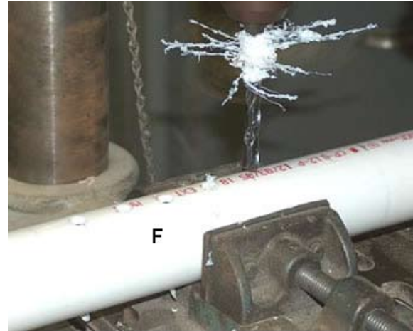
Figure 12. Drilling of ram 5/16" diameter holes in shaft (F) with 1" increments.
