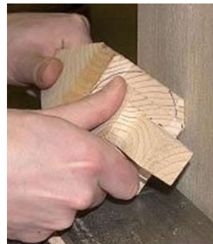
Figure 9. Sanding of dibble tip corners to reducer outer diameter.
