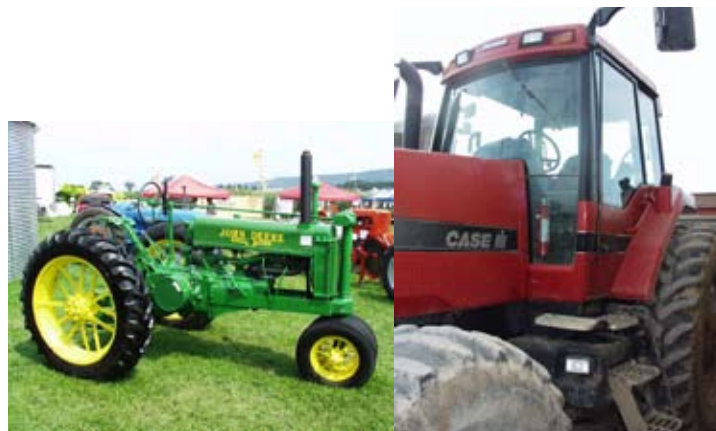
Figure 2. Older tractors expose the operator to higher noise levels than tractors with an acoustical ROPS cab.
