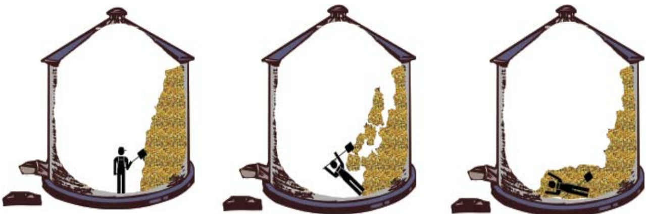
Figure 5. Avalanche of a grain wall.
