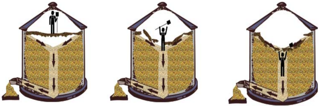
Figure 4. Collapsing grain bridge.
