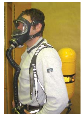
Figure 5. Supplied-air respirator (SCBA).
