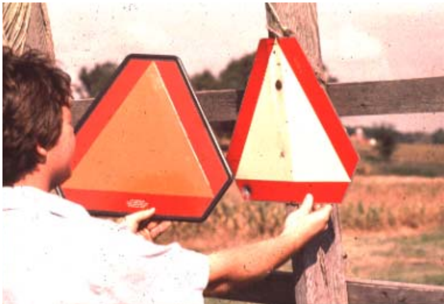
Faded and damaged SMVs should be replaced immediately with a new emblem, including one with certification as seen on the sample to the left. Please note the faded SMV emblem attached to a fence post. This is an improper use of an SMV emblem.
