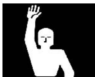
Fig 5. STOP. Raise hand upward to the full extent of the arm, palm to the front. Hold that position until the signal is understood.
