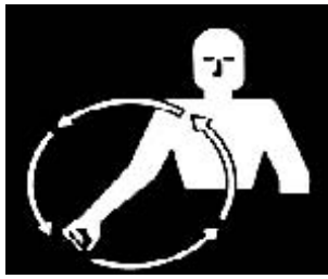
Fig 8. START THE ENGINE. Simulate cranking of vehicles by moving arm in a circular motion at waist level.
