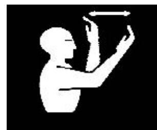
Fig 3. MOVE TOWARD ME-FOLLOW ME. Point toward person(s), vehicle(s), unit(s), beckon by holding the arm horizontally to the front, palm up, and motioning toward the body.
