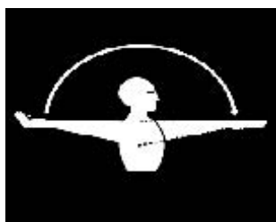
Fig 4. MOVE OUT-TAKE OFF. Face the desired direction of movement; hold the arm extended to the rear; then swing it overhead and forward in the direction of desired movement until it is horizontal, palm down.
